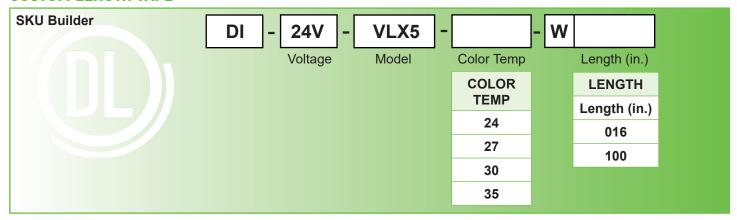
Example: DI-24V-VLX5-30-W016 = Diode LED, 24 Volt, VALENT® X, 3,000° CCT, Wet Location, 16.4 foot spool.
